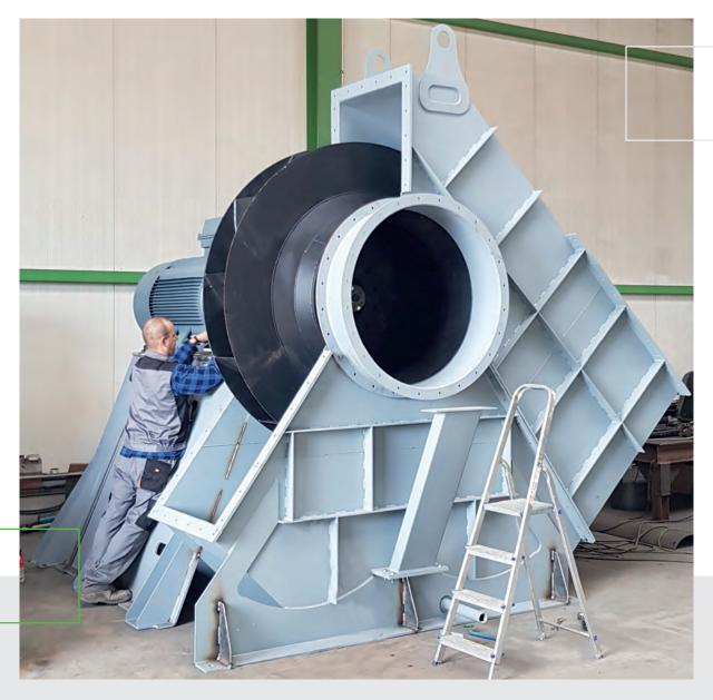
The fan housing features an internal spiral contour.
